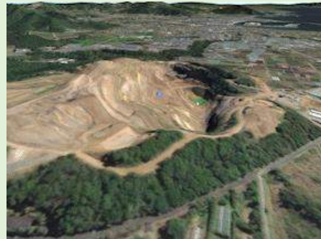
3D model of the open pit with Photogrammetry
