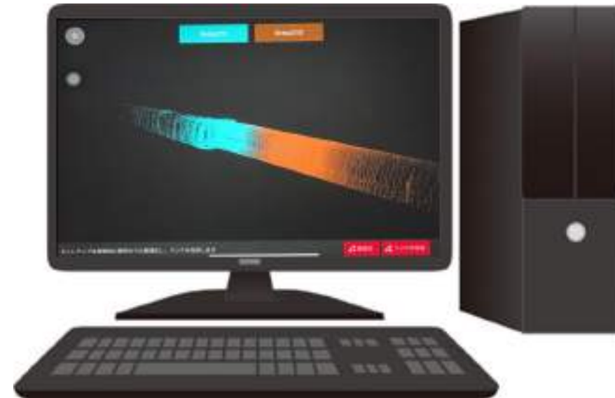
Alignment of current and previous pointcloud
