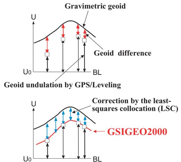
**Fig. 4** Schematic diagram of hybrid geoid model construction.
