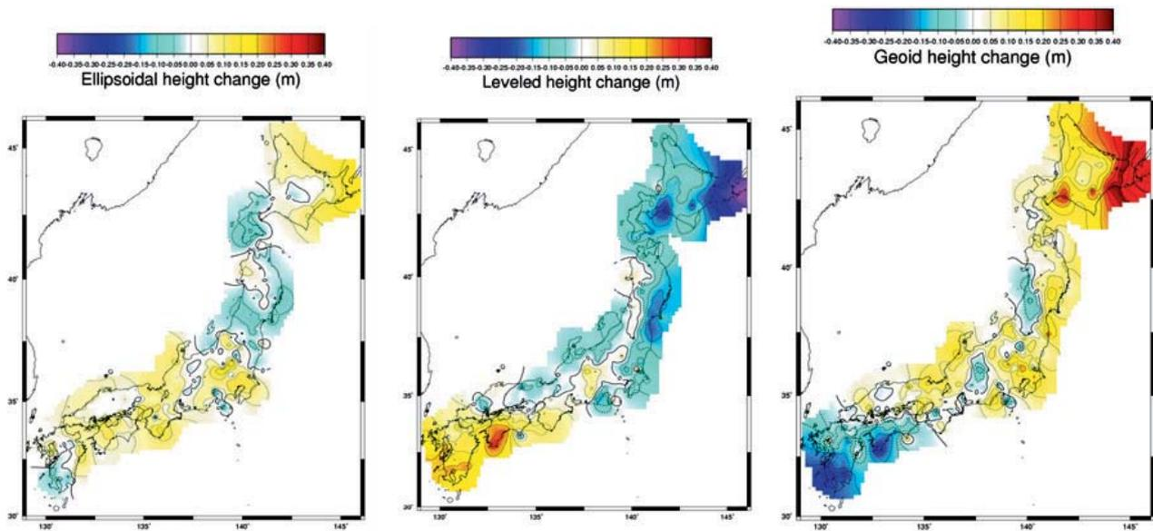
**Fig. 3** The difference between the old and new analyses for GPS ellipsoidal heights (left), leveled heights (middle) and geoid undulation data (right). Color scale is  $-0.4\text{m}$  to  $0.4\text{m}$ . Contour interval is  $5\text{m}$  and broken lines show contours of negative value.
