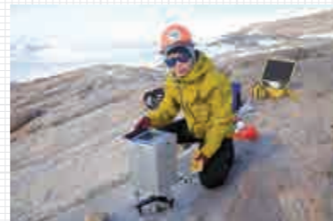
Taking relative gravity measurements on an outcrop (photo taken during the 62nd mission)
