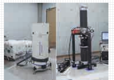
(Left) AQG Absolute quantum gravimeter (Right) FG5 Absolute gravimeter
