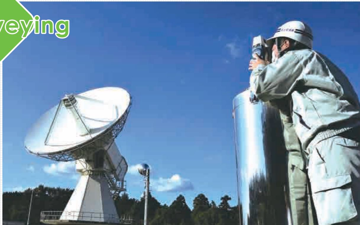
The position of the center of the VLBI antenna is measured in order to establish accurate position references (Ishioka VLBI observing facility in Ishioka City, Ibaraki Prefecture)
