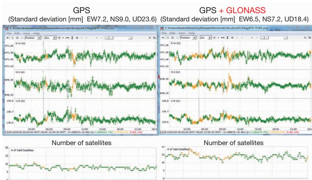
**Fig.8** Time series of kinematic baseline analysis between GEONET stations (Onoda to Shikama, distance 11 km) for 1 day. Left: GPS only. Right: GLONASS is used together. Minimum elevation angle is 15°.
