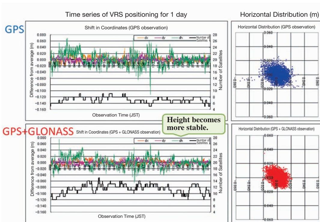
**Fig.11** Example of network-based RTK performance with GLONASS. One day time series using Jenoba’s Virtual Reference Station method (VRS). Minimum elevation angle is 15°. (Promotion Council of Real Time Positioning using GPS-based Control Stations, 2013, p.24, modified)
