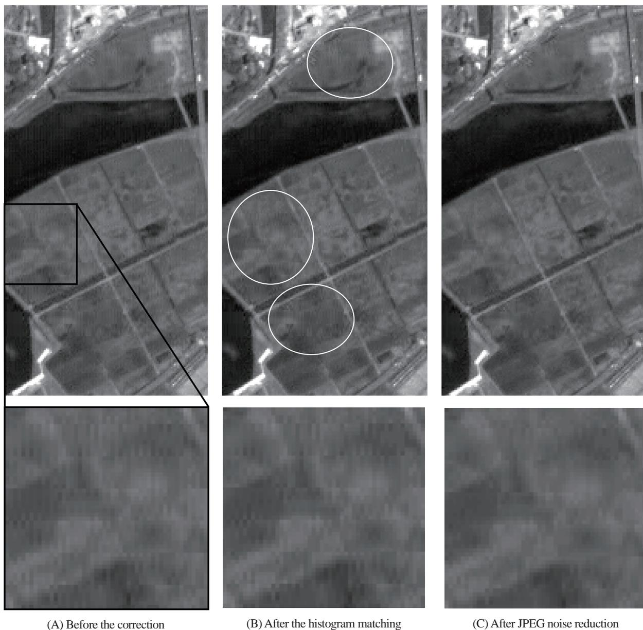
**Fig.3** Result of JPEG Noise Reduction (focusing on block noise, part of the Nagasaki scene)
